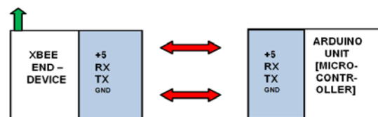
Fig. 4. XBEE and ARDUINO [MICROCONTROLLER UNIT] interfacing at ARDUINO UNIT end.
