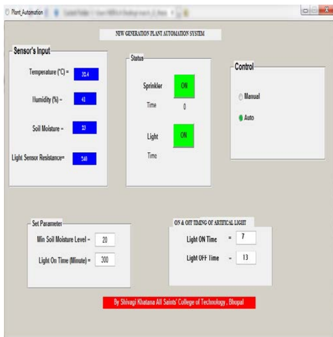
Fig. 6. GUI of NEW GENERATION PLANT AUTOMATION SYSTEM
