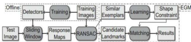
Fig.5 Pipeline of the proposed system for detecting facial landmarks [27]
