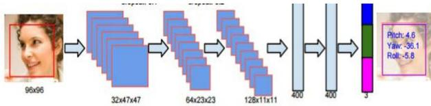
Fig.7 Convnet model for head pose estimation [10].
