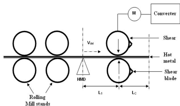
Figure 1 Principle of Operation of Shear
