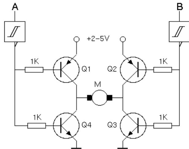
Figure.5.Arrangement of H-Bridge
