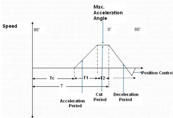
Figure 2 Speed Time Characteristics of Start-Stop Shear
