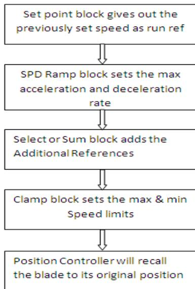
Figure 4.Speed Reference Block
