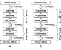
Fig.1. Encryption and Decryption block diagram
