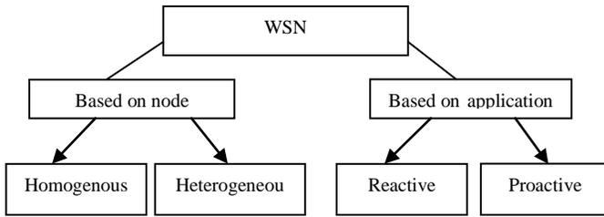
Figure 2:Types of Wireless sensor networks
