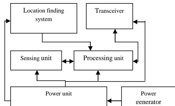
Figure 1: Sensor node components
