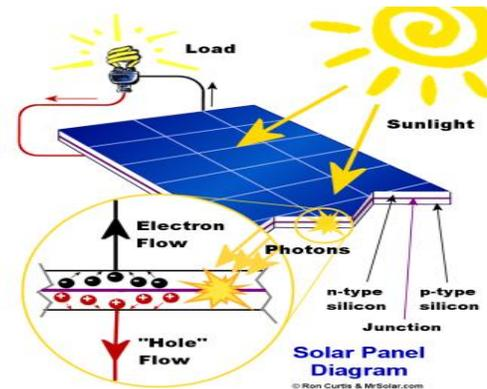
Fig 1. Simple process flow in solar panel
