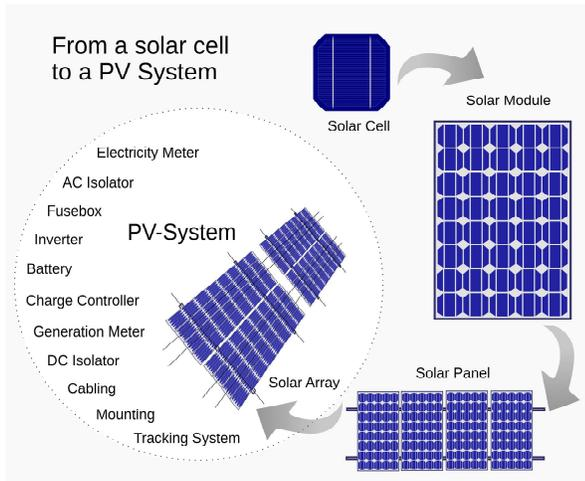
Fig 2. Elements in Electricity generation
