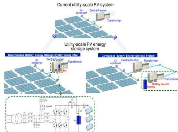
Fig 4. Utility-Scale PV-Energy Storage Systems with the Single Stage Inverter cum Chopper (SSICC) and the Current State-of-the-art Solution
