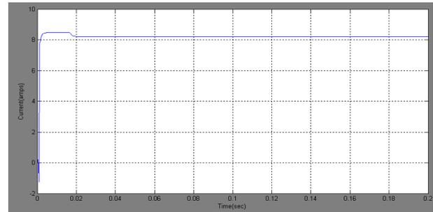
Fig 8.6 PV Output Current for DC-DC Converters ion
