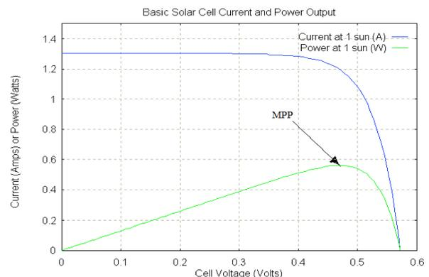
Fig.7.1 PV Module Power/Voltage/Current Characteristics
