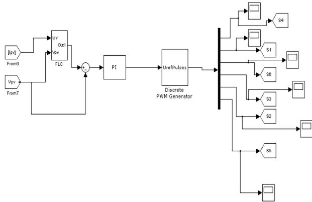
Fig 8.4 Simulink Model of FLC Block For DC-DC Operation
