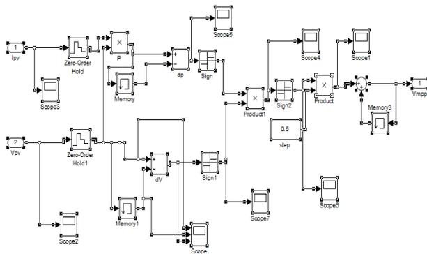
Fig 8.1 Simulink Model of MPPT
