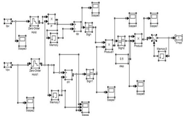
Fig 8.2 Simulink Model of MPPT Controller Block For DC-AC Operation
