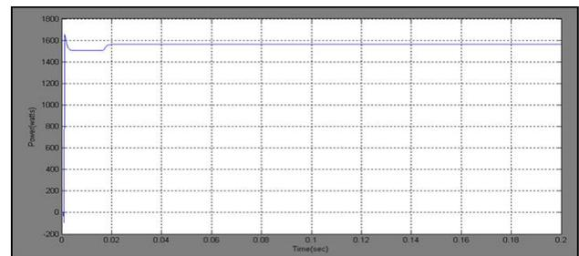
Fig 8.7 PV Output Power for DC-DC Converters ion
