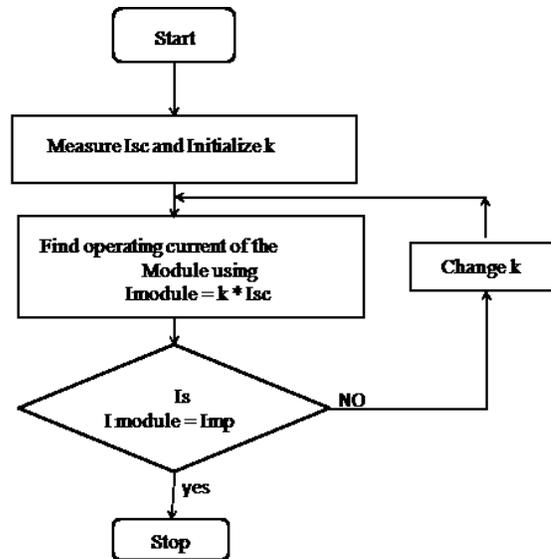
Fig 7.3 Flow Chart For the Short-Circuit Method
