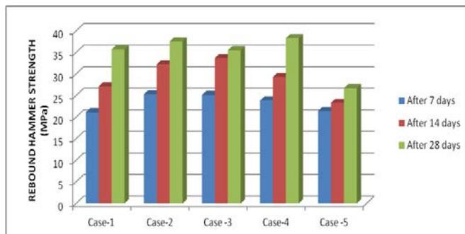
Figure 10: Average Rebound Hammer Compressive Strength
