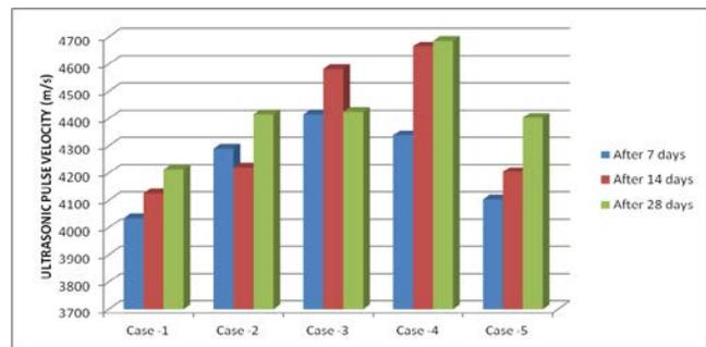
Figure 11: Average Ultrasonic Pulse Velocity Values
