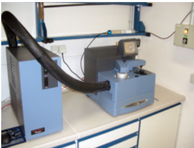
3.9 Four Ball wear Tester
