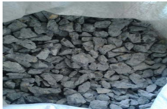
Fig 2. Recycled Coarse aggregates after Crushing and sieving
