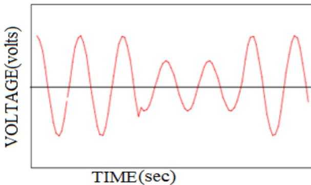
Fig. 2 Voltage sag- Reduced voltage for limited time period
