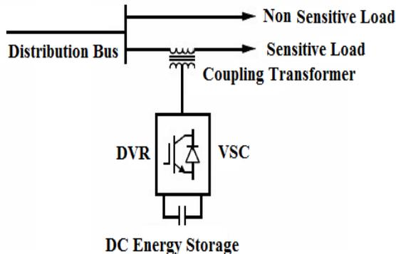
Fig. 4 Basic arrangement of DVR
