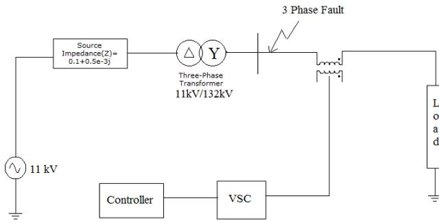
Fig. 8 Single Line Diagram of Test System
