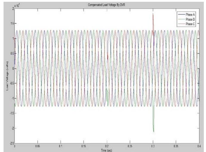
Fig. 11 Compensated Load voltage with DVR
