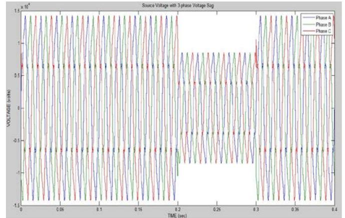
Fig. 10 Source voltage with 3-phase sag
