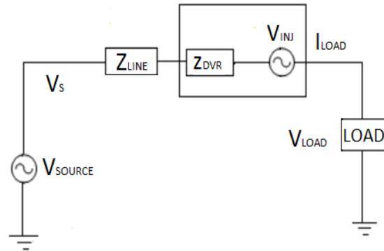
Fig. 5 Equivalent circuit diagram of DVR
