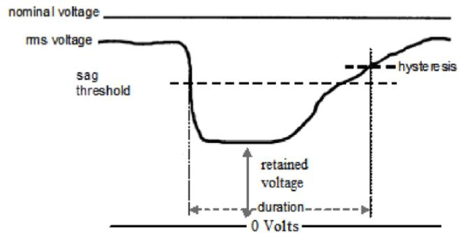
Fig. 3 Example of voltage sag
