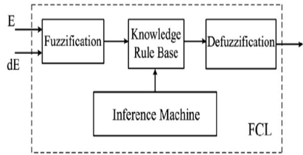
Fig. 6 Block diagram of fuzzy logic controller
