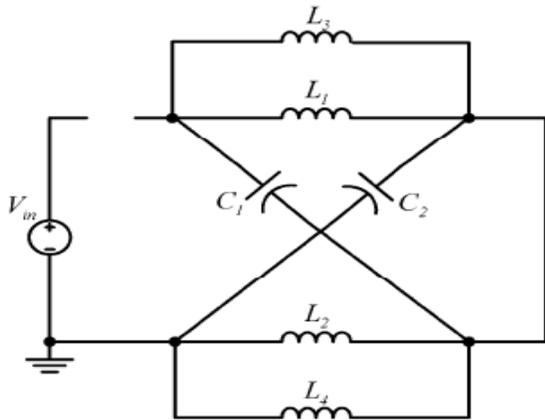
Fig.2. Equivalent circuits: Shoot-through zero state (switching-on).
