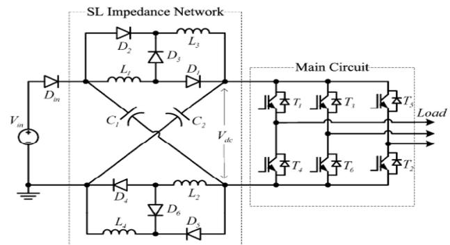
Fig.1. Proposed SL Z-source inverter.
