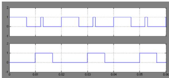
Fig.7. Driving Pulses for first leg.
