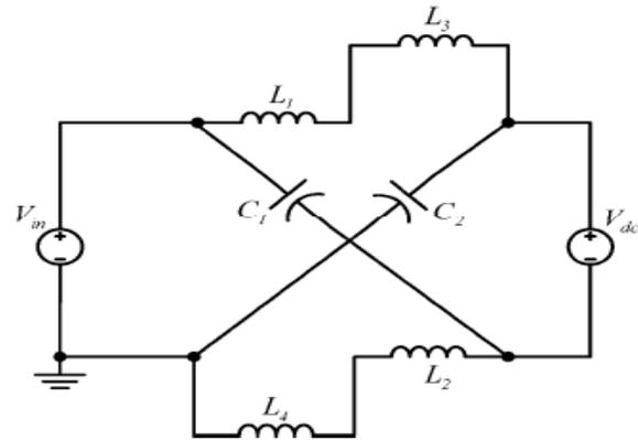
Fig.3. Equivalent circuits: Non-shoot-through states (switching-off).
