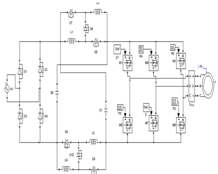
Fig.4. Proposed SL Z-source inverter fed Induction Motor.
