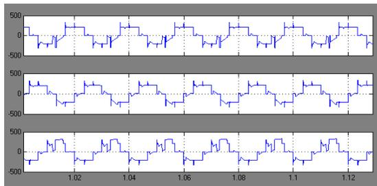
Fig.8. Phase to Phase Output Voltage.
