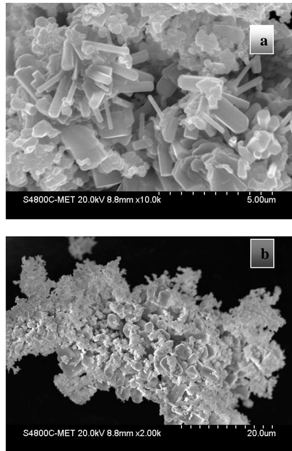
Fig. 2. FESEM images (a) and (b) correspond to heated admixture of PPS and zinc nitrate in molar ratio of 1:1
