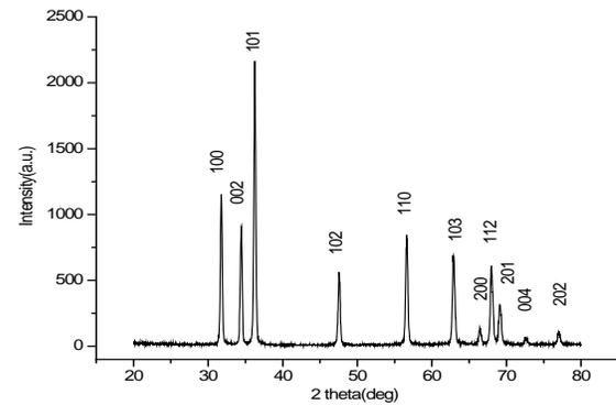
Fig. 1. X-ray diffractogram correspond to heated admixture of PPS and zinc nitrate in molar ratio of 1:1.
