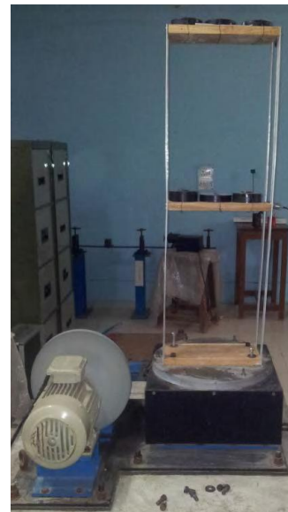
Fig. 2.1. Experimental setup for two-story building frame.
