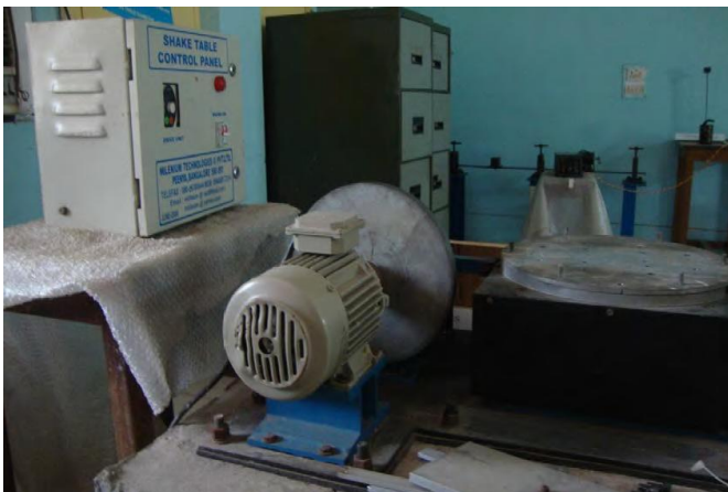
Fig. 1.2. Electro-dynamic 30Kg-f shake table.
