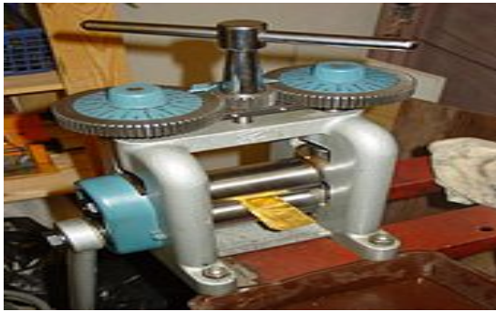
Fig .3: Rolling mill for cold rolling with metal piece of brass sheet.
