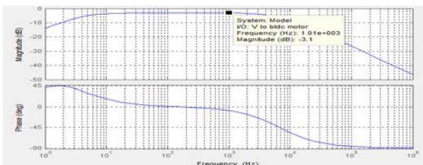
Fig5.2 current loop (closed)
