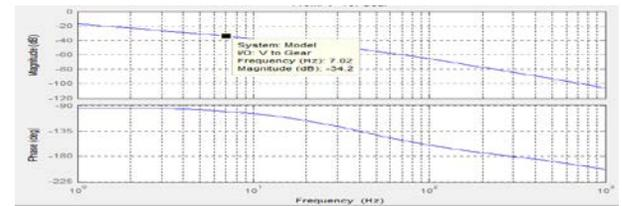
Fig5.13 position loop (open)
