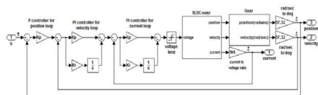
Fig4.1. Current, velocity and position loop controller model
