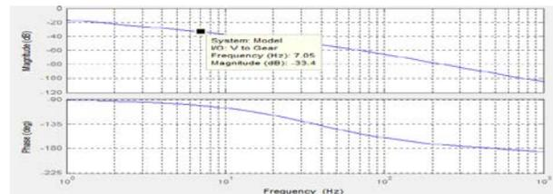
Fig5.5 position loop (open)
