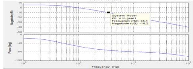
Fig5.11 velocity loop (open)
