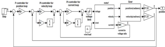
Similarly now adding the disturbance, the wind load effect and their respective time responses are plotted for a step input of 1°/sec.
