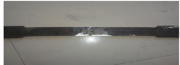
Fig03: MIG welded piece after breakage
