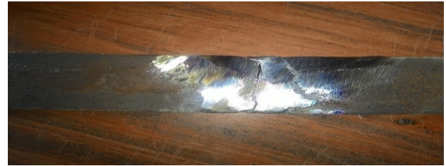
Fig02: Gas welded piece after breakage
