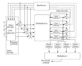
Fig 7 Turbo-BLAST iterative detection and decoding scheme
