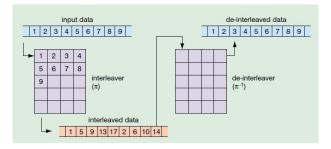
Fig 8. Operation of interleaver and de-interleaver
