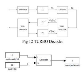
Fig 13 RSC feeds the decoder by the systematic ri and the parity bit rp
