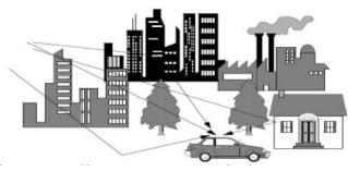
Fig 1 Multipath Propagation
