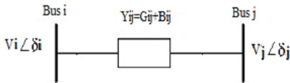
Fig 4.2 Model of transmission line without TCSC
