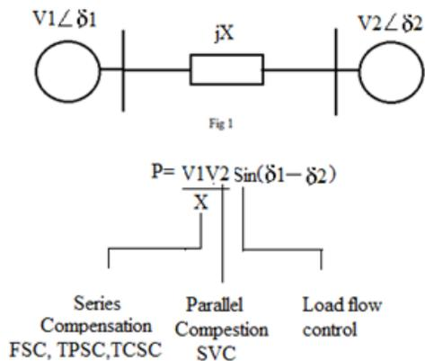
Fig 2.1 Active power transmission equation
