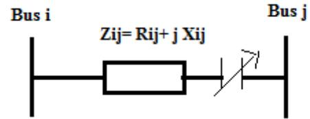
Fig 4.3 Model of transmission line with TCSC
