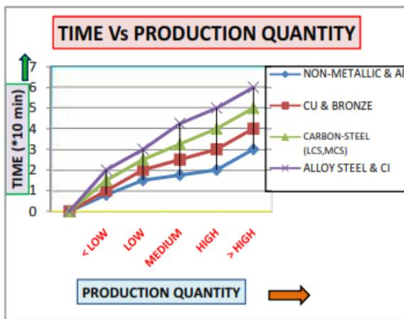
The graphical analysis is provide to conditions of carbide form tool material, spur type gear teeth form, total depth is 6mm. in the productivity is increases for softened as low time consuming possibility. But, hard and brittleness materials to take more time consuming for production quantity to increasing possibility.
