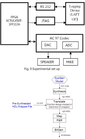
Fig. 10 Flow of .bit file Generation
