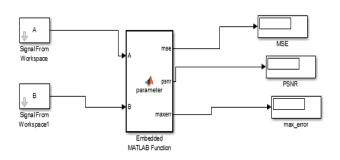
Fig.11 MATLAB Simulink Model for Parameter Evaluation
