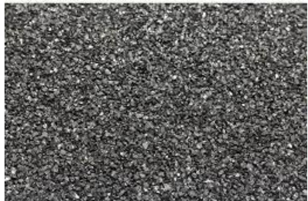
Figure 07 Copper Slag
