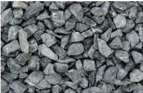
Figure 04 Coarse Aggregates
