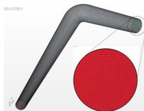
Figure 3 Geometry and meshing employed for the elbow pipe bend.
