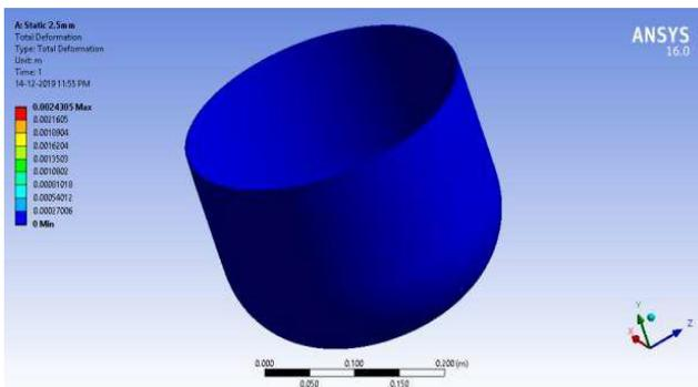
**Fig.4.11** Total Deformation of Steel LPG cylinder (2.5mm)
