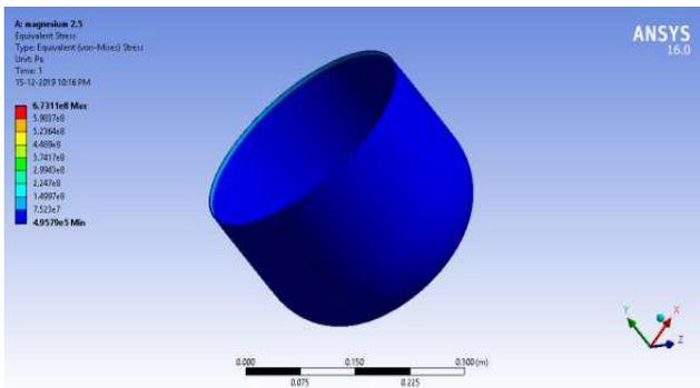
**Fig.4.10** von Mises stress of Magnesium LPG cylinder (2.5mm)
