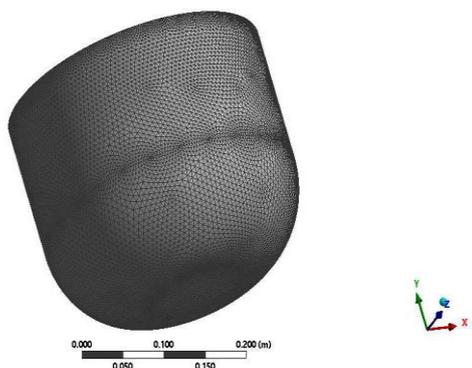
Fig.4.5 Mesh Model of LPG cylinder
