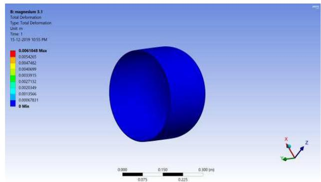
**Fig.4.25** Total Deformation of Magnesium LPG cylinder (3.1mm)
