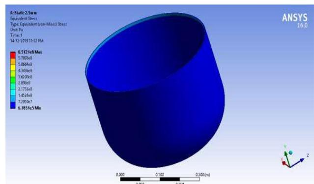
Fig.4.8 von Mises stress of Steel LPG cylinder (2.5mm)
