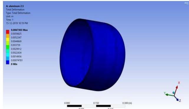
**Fig.4.12** Total Deformation of Aluminum LPG cylinder (2.5mm)
