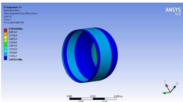
**Fig.4.22** von Mises stress of Magnesium LPG cylinder (3.1mm)
