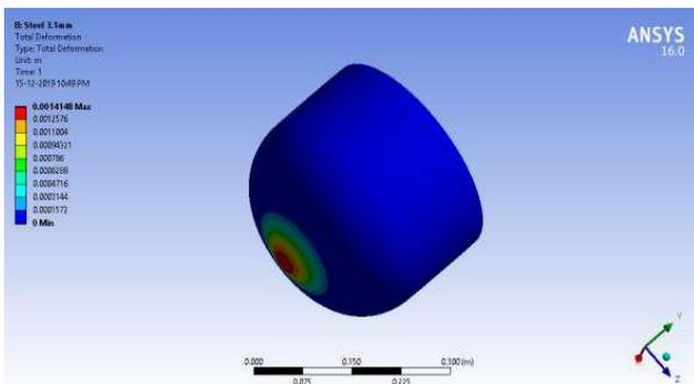
**Fig.4.23** Total Deformation of Steel LPG cylinder (3.1mm)
