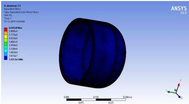
**Fig.4.9** von Mises stress of Aluminum LPG cylinder (2.5mm)
