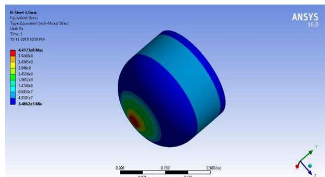
**Fig.4.20** von Mises stress of Steel LPG cylinder (3.1mm)
