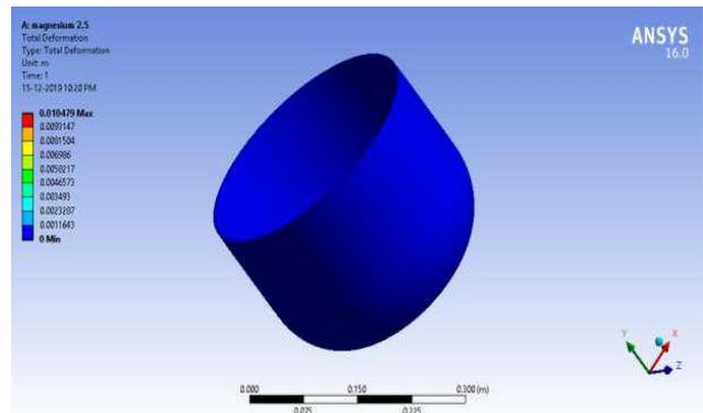
**Fig.4.13** Total Deformation of Magnesium LPG cylinder (2.5mm)
