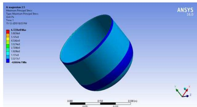
**Fig.4.19** Maximum principal stress of Magnesium LPG cylinder (2.5mm)
