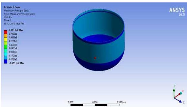
**Fig.4.17** Maximum Principal Stress of Steel LPG cylinder (2.5mm)
