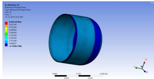
**Fig.4.18** Maximum principal stress of Aluminum LPG cylinder (2.5mm)
