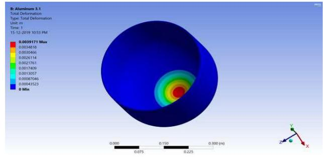
**Fig.4.24** Total Deformation of Aluminum LPG cylinder (3.1mm)
