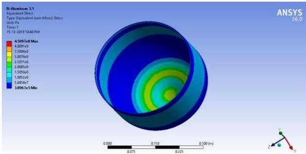
**Fig.4.21** von Mises stress of Aluminum LPG cylinder (3.1mm)
