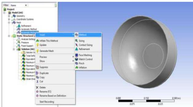
Fig.4.3 Inserting the method of meshing
