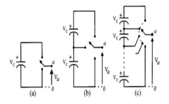
Figure 1.One phase leg of an inverter with (a) two levels, (b) three levels, and (c) n levels. Semiconductors is represented by an ideal switch with several positions.
