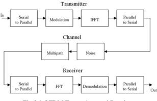
Fig.2.1 OFDM Transmitter and Receiver
