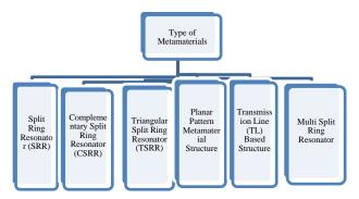
Figure 2. Various Metamaterial Structures.
