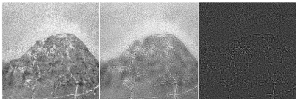
a) Noisy SAR_image_3 b) Lee filtered SAR Image c) Kuan Filtered image
