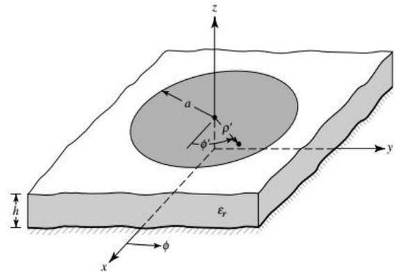
**Figure 1.** Basic circular patch antenna.
