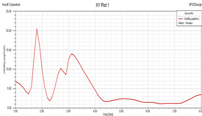
Figure.10 : VSWR of simulation result for Design 3.
