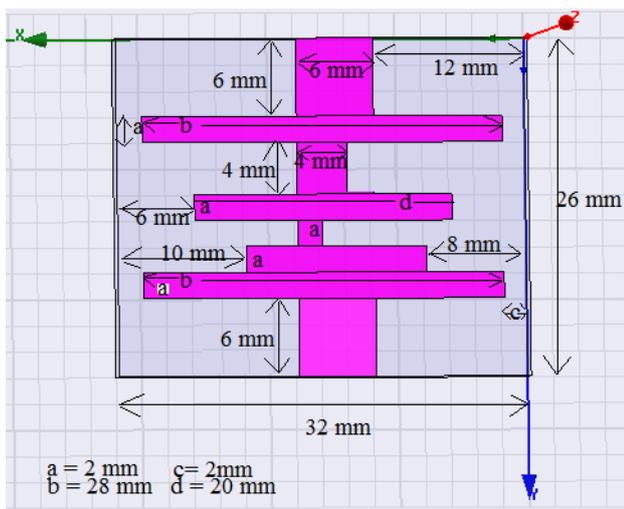
Figure.2 Top view of Second SIR Design model.
