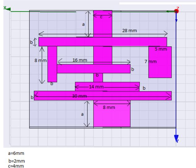
Figure.3 Top view of Third SIR Design model with suspended Impedance Line.
