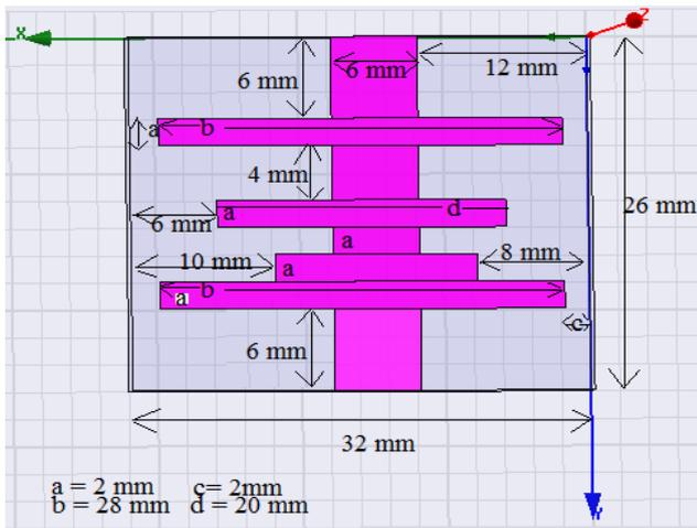
Figure.1 Top view of First SIR Design model.
