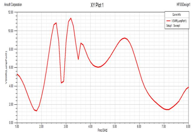
Figure.7 : VSWR of simulation result for Design 2 .
