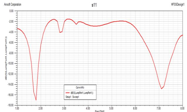
Figure.6 : Return loss of simulation result for Design 2.
