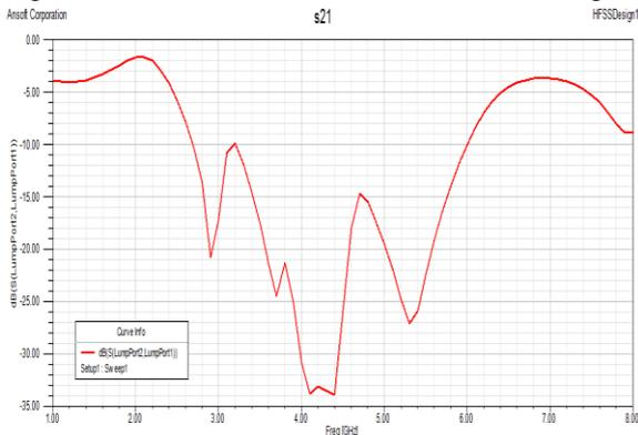
Figure.5 : Insertion Loss for simulation result for Design 1
