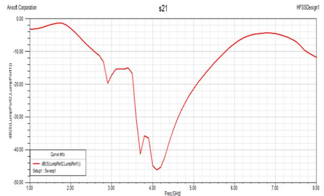
Figure.8 : Insertion Loss of simulation result for Design 2.
