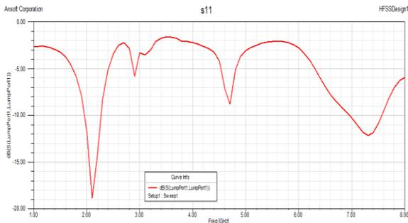
Figure.3 : Return loss for simulation result for Design 1
