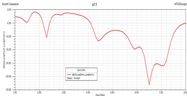
Figure.9 : Return loss of simulation result for Design 3.
