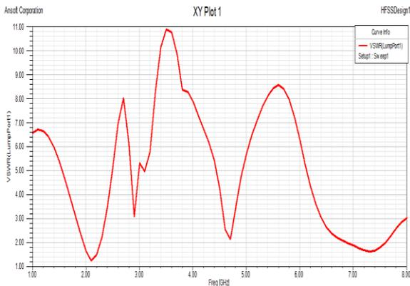
Figure.4 : VSWR for simulation result for Design 1
