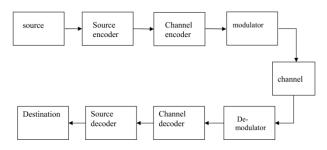
Figure: 1.1 Functional Block in a Communication System.
