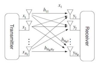
Fig.2.1 N<sub>R</sub> X N<sub>T</sub> MIMO System
