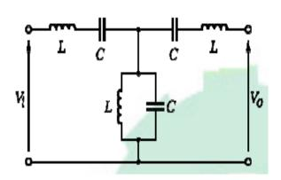
Figure 3: Band pass filter circuit
