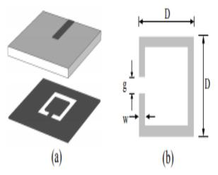
Figure 2: DGS resonator configuration
