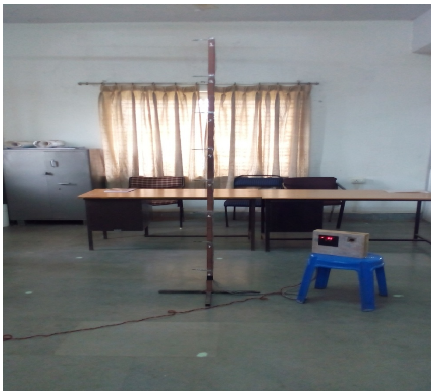
Figure 1 : Experimental Model ,Thermocouples connected in series with ammeter for measuring temperature
