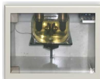
Fig. 1. Laboratory oil tester testing device of oil discharge decomposition.
