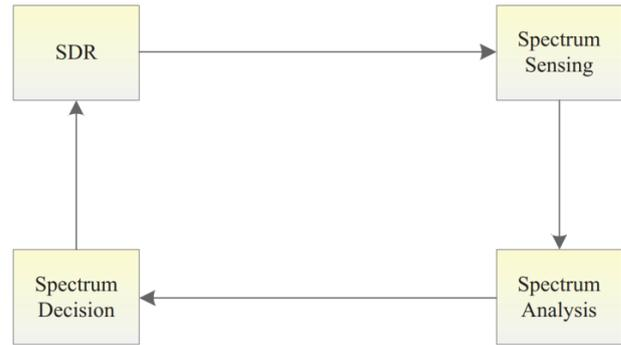
Fig. 2.1A concept diagram of cognitive radio (CR) showing the basic procedure performed by CR.
