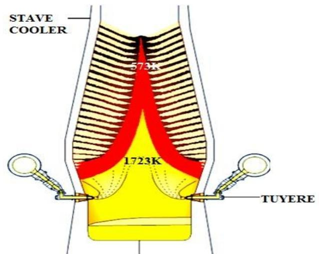
Thermal Zone of Blast Furnace
