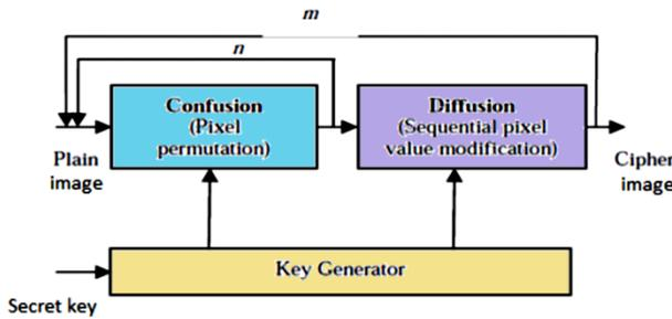
Figure 2.1 Chaos Based image encryption systems.
