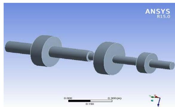
Shaft with Variable Diameter diameter (70-100) and Different Materials
