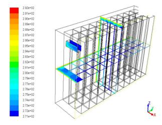
Above fig is showing the temperature distribution for case 2 at the middle section of chamber. It is clear from the fig that there is less uniformity of temperature in the above case along both height and length of the chamber.
