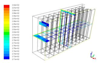
Above fig is showing the temperature distribution for case 1 at the middle section of chamber. It is clear from the fig that there is uniformity of temperature in the above case along both height and length of the chamber.
