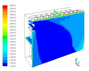
Above fig shows the temperature distribution of cold chamber having an evaporator in which the direction of flow of air is vertically downward and after reflecting with the plate, flow along the length of the chamber air is not reaching up to the end wall of the cold chamber. Temperature distribution is also not uniform. Hence heat transfer will be less which results in poor performance of the machine.
