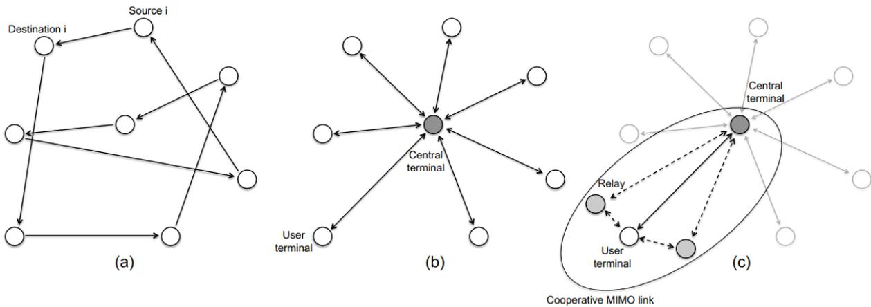
Figure 1.2 Models for (a) ad-hoc network configuration with n source-destination node pairs, (b) star network configuration with one central terminal (shaded) and n user terminals, and (c) cooperative link as a part of star network configuration.
