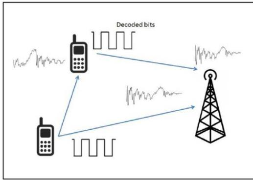
Figure 2.1 Decode and Forward (DF) Relaying Scheme.
