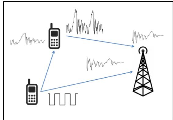
Figure 2.2 Amplify and forward relaying Scheme.
