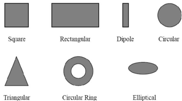
Figure 1.2 Different Shapes of patch elements.
