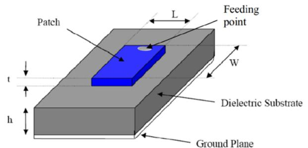
Figure 1.1 Basic Structure of a microstrip patch antenna.
