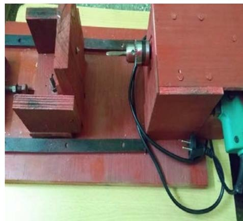
Fig-2.3 mini lathe top view (showing head stock, tail stock, chuck, motor)
