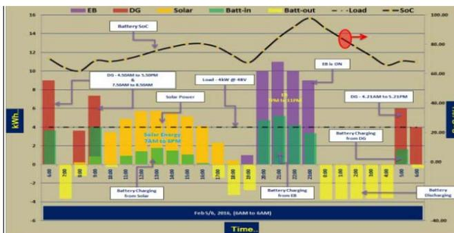
Fig 2 System profiling for single day with 4 hrs of grid availability
