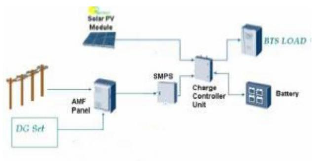
Fig.1 Solar Present, Grid available Battery Charged through MPPT charge + main Load supplied through Grid
