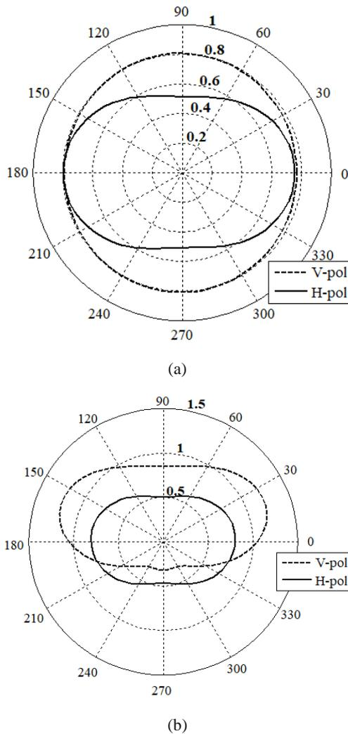
Fig.5. Polar plots showing the circularity of the H-pol and V-pol components of the electric field patterns of the SSD (a) without the tower and (b) with the tower.
