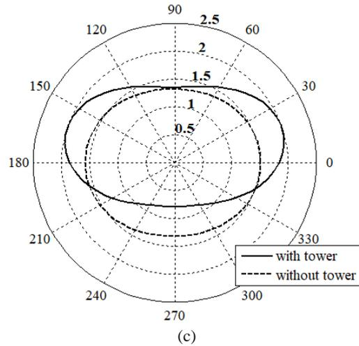
Fig.4. Polar plots of the gains of the SSD with and without the tower to illustrate the tower effects on the pattern circularity of the (a) H-pol component, (b) V-pol component patterns and (c) total gain patterns.
