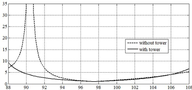
Fig.3. Standing Wave Ratio of the SSD with and without the tower over the entire FM band.
