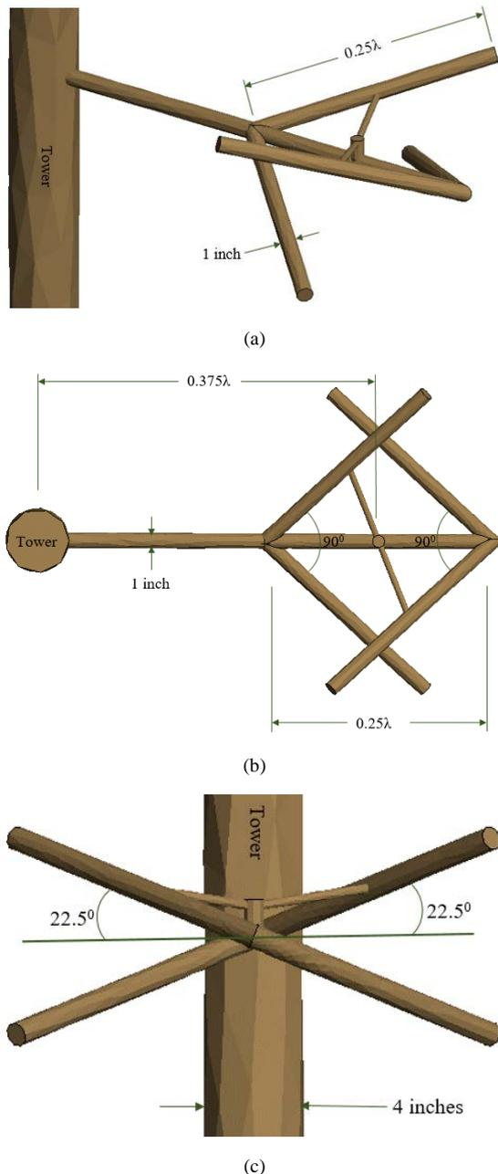
Fig.2. Computer rendition of the SSD in different views: (a) isometric, (b) top and (c) front. The SSD is side-mounted to the center of a metallic tower one wavelength long.
