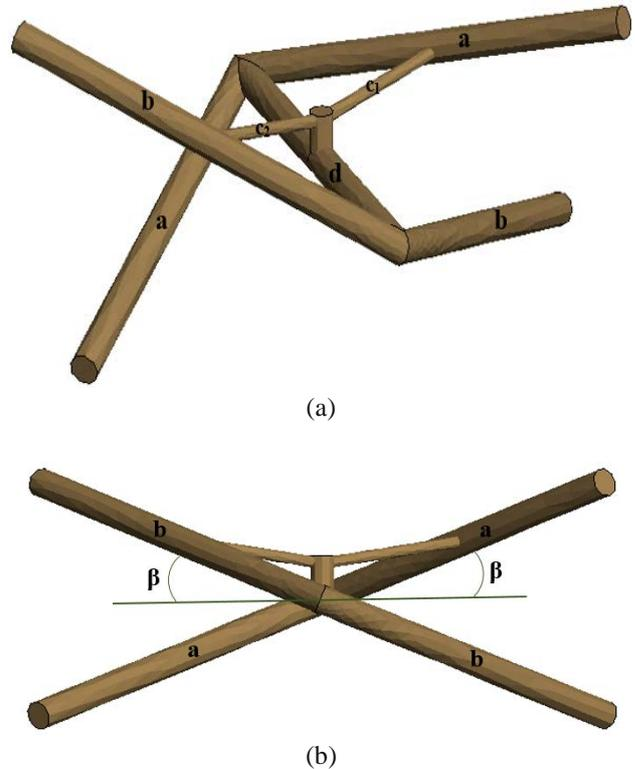
Fig.1. The Shunt-fed, slanted dipole in (a) Isometric view and (b) Front view showing the different parts and specifications: a - arms of the first dipole; b - arms of the second dipole; c<sub>1</sub>, c<sub>2</sub> – feed arms of the first and second dipoles, respectively; d – boom;  $\beta$  – skew angle.
