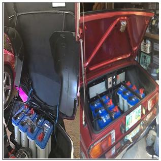
Figure B. Ten 12-volt batteries Creating the Conversion
