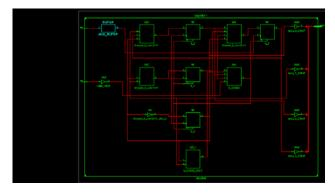
Figure 5 : Schematic design of counter with Synchronous reset
