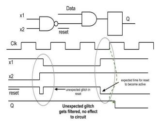
Figure 2 : Glitch with synchronous reset
