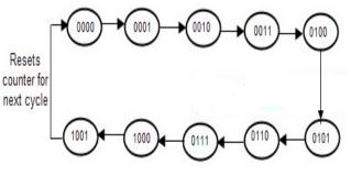
Figure 1: BCD Counter State Diagram
