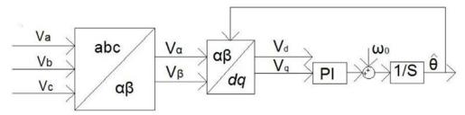
Figure: 2.1. Basic Block Diagram of the Conventional PLL.
