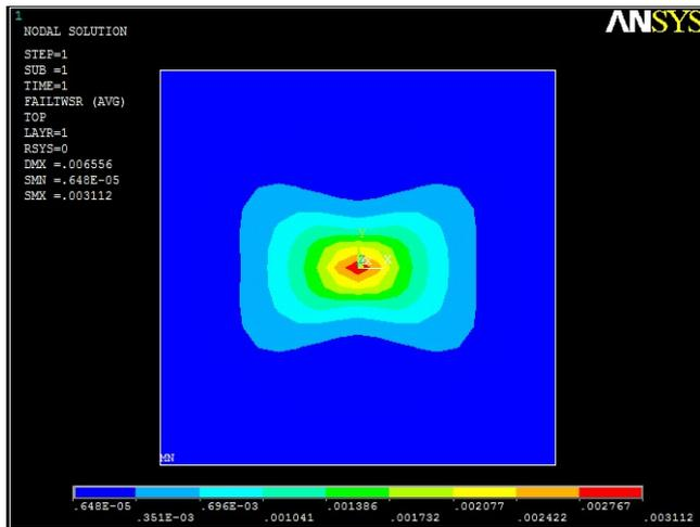
Fig. 9 Tsai-Wu failure index for  $(0^\circ/90/0^\circ/90)_s$  laminates
