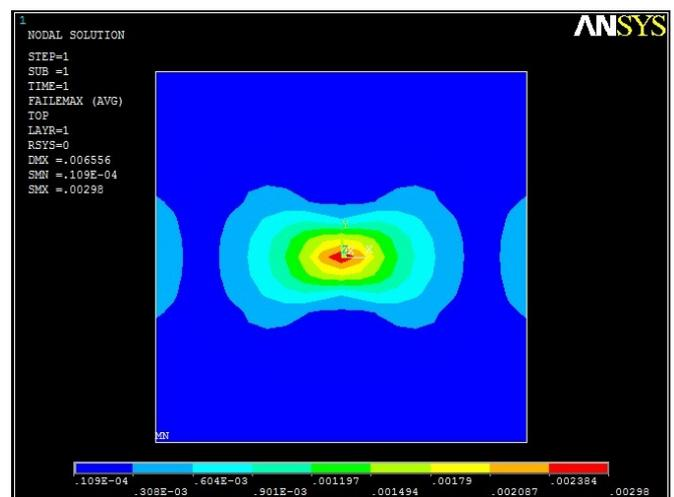
**Fig. 8 Maximum Strain failure index for  $(0^{\circ}/90^{\circ}/0^{\circ}/90^{\circ})_s$  laminates**
