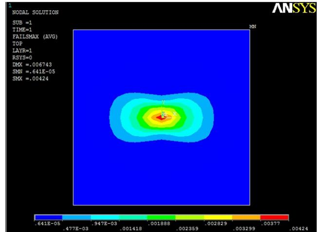
Fig. 3 Maximum Stress failure index for  $(0_2/90_2)_s$  laminates
