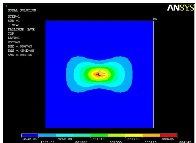
Fig. 5 Tsai-Wu failure index for  $(0_2/90_2)_s$  laminates
