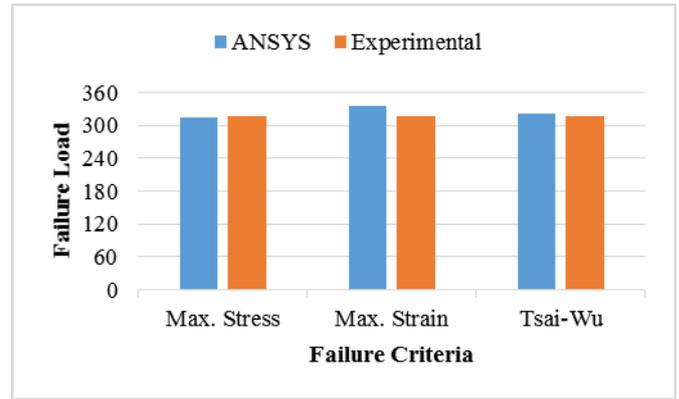
**Fig. 6 Comparison of ANSYS and Experimental results for  $(0^{\circ}/90^{\circ}/0^{\circ}/90^{\circ})_s$  stacking sequence**
