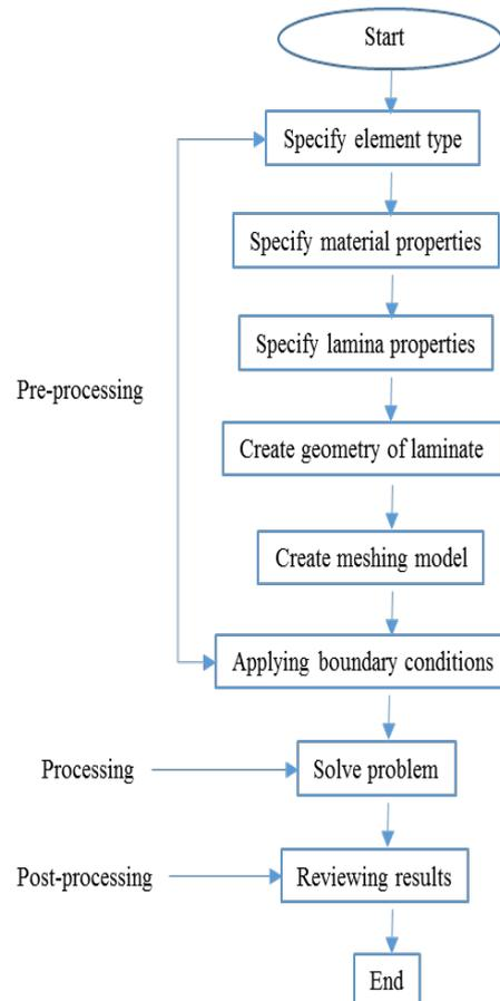
Fig. 2 flow chart for simulation process
