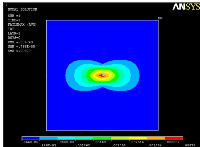
Fig. 4 Maximum Strain failure index for  $(0_2/90_2)_s$  laminates
