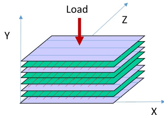
Fig.1 Stacking sequence for (0°/90°/0°/90°)s plates
