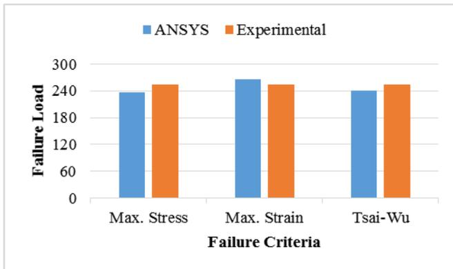
Fig. 2 Comparison of ANSYS and Experimental results for  $(0_2/90_2)_s$  stacking sequence
