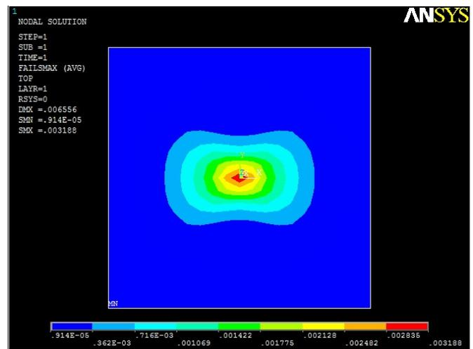
**Fig. 7 Maximum Stress failure index for  $(0^{\circ}/90^{\circ}/0^{\circ}/90^{\circ})_s$  laminates**
