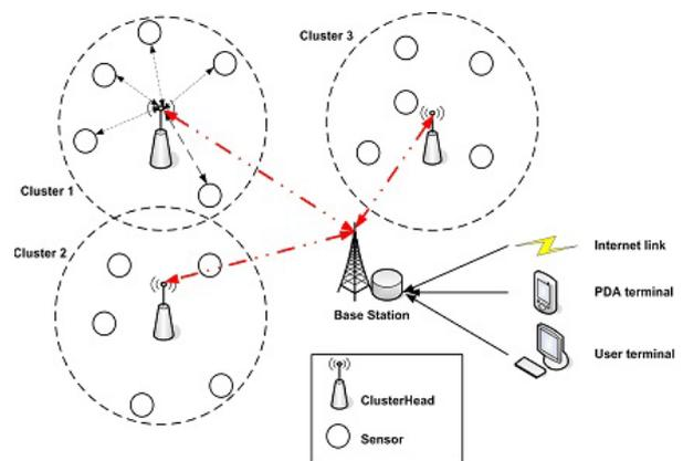
Figure 2.1 Clustered Sensor Network.
