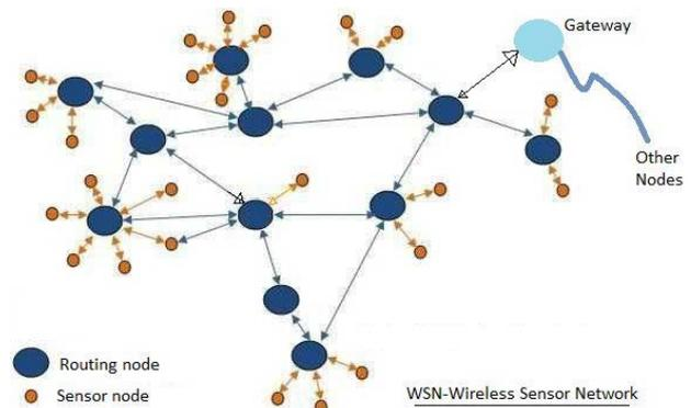
Figure 1.1 wireless Sensors Network
