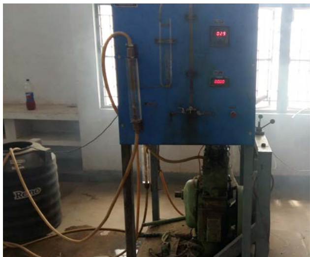
Fig.3 Single Cylinder 4-Stroke Engine with Rope Brake Dynamometer
